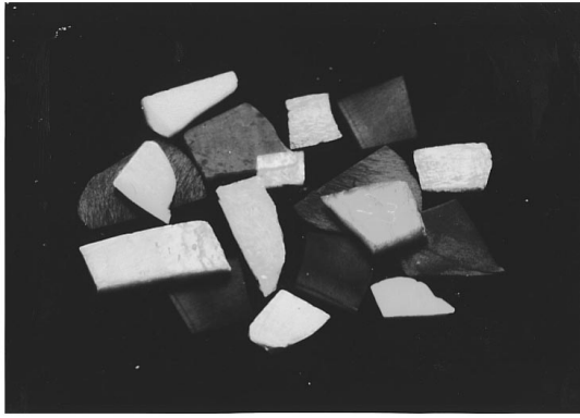
FIG. 1. A set of opal samples with axes oriented at different angles with respect to the incident light direction (in water).
